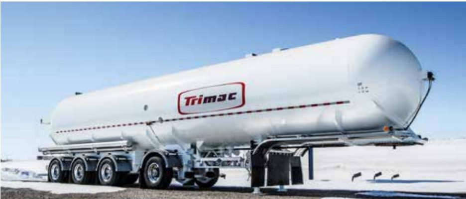
19,300 GALLON - LP - TRI-AXLE WITH LIFT
