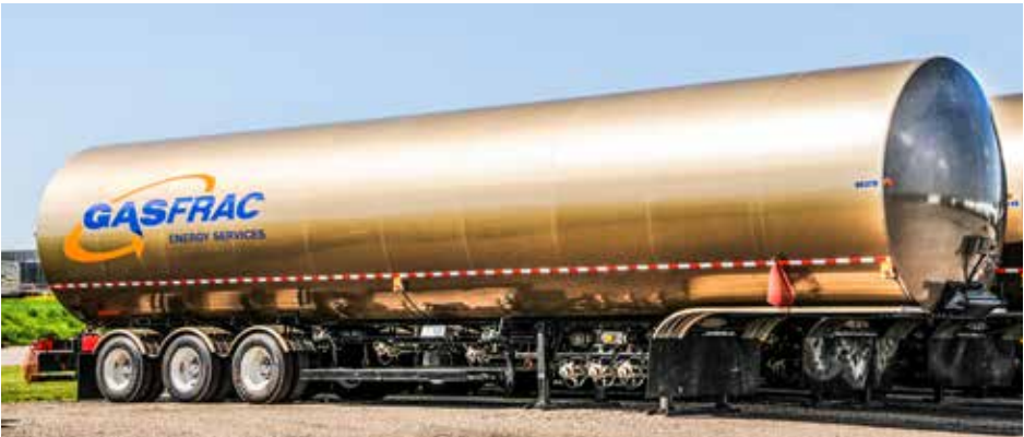
23,200 GALLON - LP - 350 PSI - PORTABLE STORAGE
