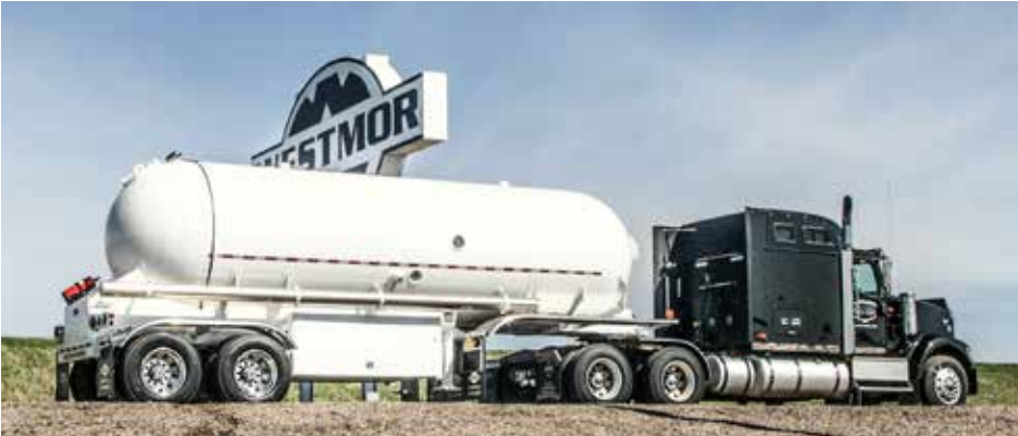
7,000 GALLON - NH 3 - 80" DIAMETER - METERED DELIVERY
