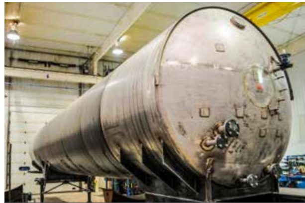
STAINLESS STEEL INNER VESSEL
