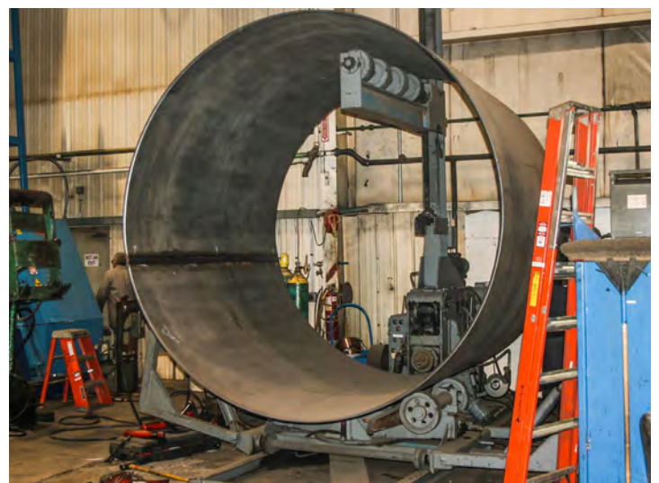
IN-HOUSE TANK ROLLING
