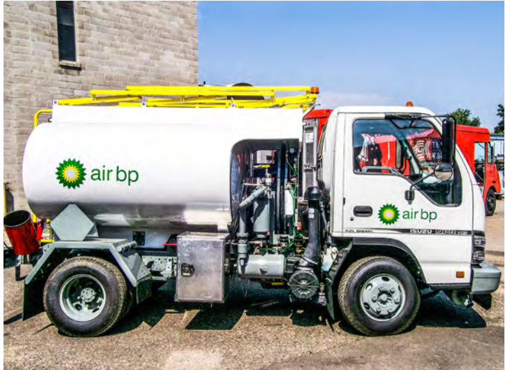
1,000 GALLON AVGAS / MID MODULE
