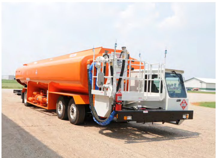
10,000 GALLON JET REFUELER WITH LIFT DECK
