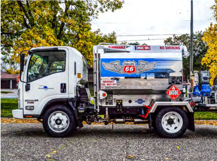
1,000 GALLON AVGAS / REAR MODULE
